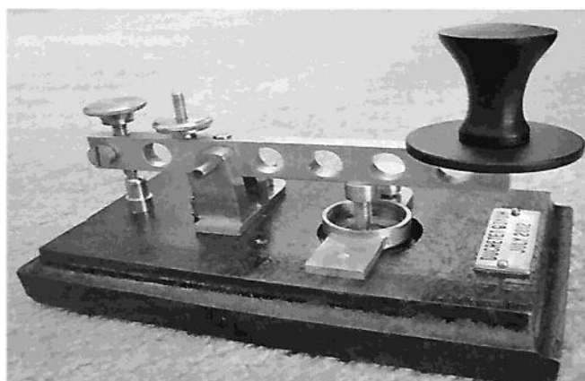
↑ The G3YUH copy of the Ducretet oil-break flameproof key without the oil cup lid in place.
