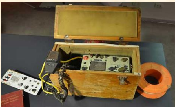
Restored Traeger Receiver, VNJ-88, with Daryl's Traeger Scout front panel at the left. The orange reel contains the aerial wire for the transceiver.
