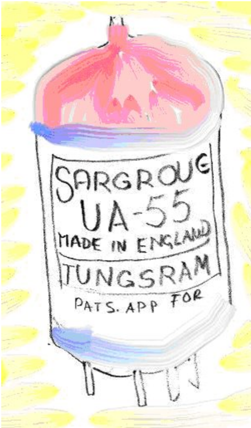
Picture 2. The basis of Sargove radio was a general tube, UA-55, which fit every purpose sufficiently well. There were two tube functions in the same envelope.
