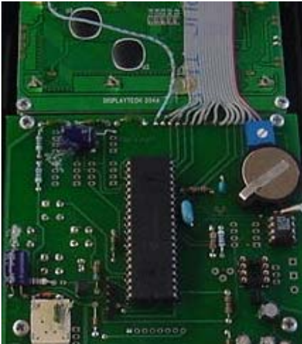
Picture 12 Two sided through coppered circuit plate with LCD and processor
