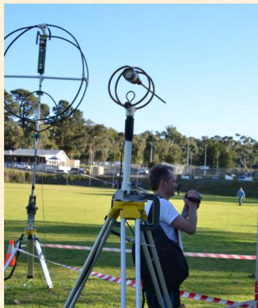
◀◀ Steve's 160m and 6m TMLA loops at the WIA Convention weekend. Note that these are double loops.
