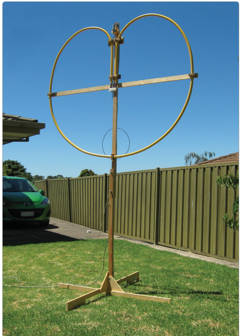
Photo 1: The completed magnetic loop.
