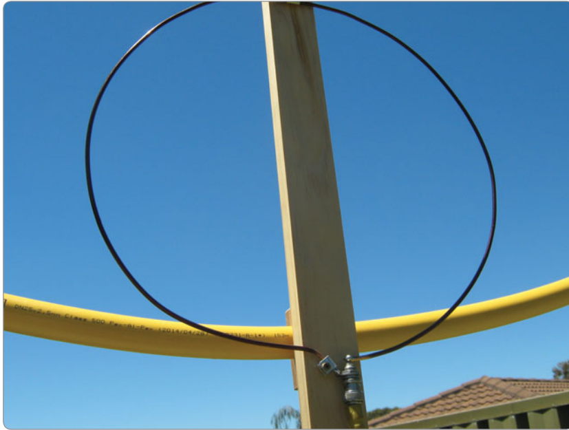
Photo 5: The copper wire driving loop.
