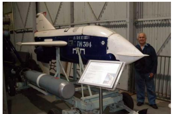
Mark, VK5AQV, standing by an Ikara missile, a small missile which carried an anti-submarine torpedo. The missile was developed here in Adelaide, at our DSTO facility.
